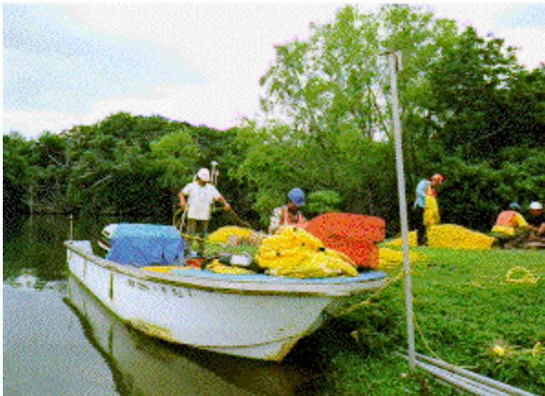
Swift Energy seismic survey in Fayette County, Texas. A crew prepares to precisely position hydrophones on the bottom of Fayette Lake to detect seismic signals. Yellow cables link the hydrophones to electronics encased in the orange boxes, which will float on the lake surface and transmit signals to a nearby recording truck.
